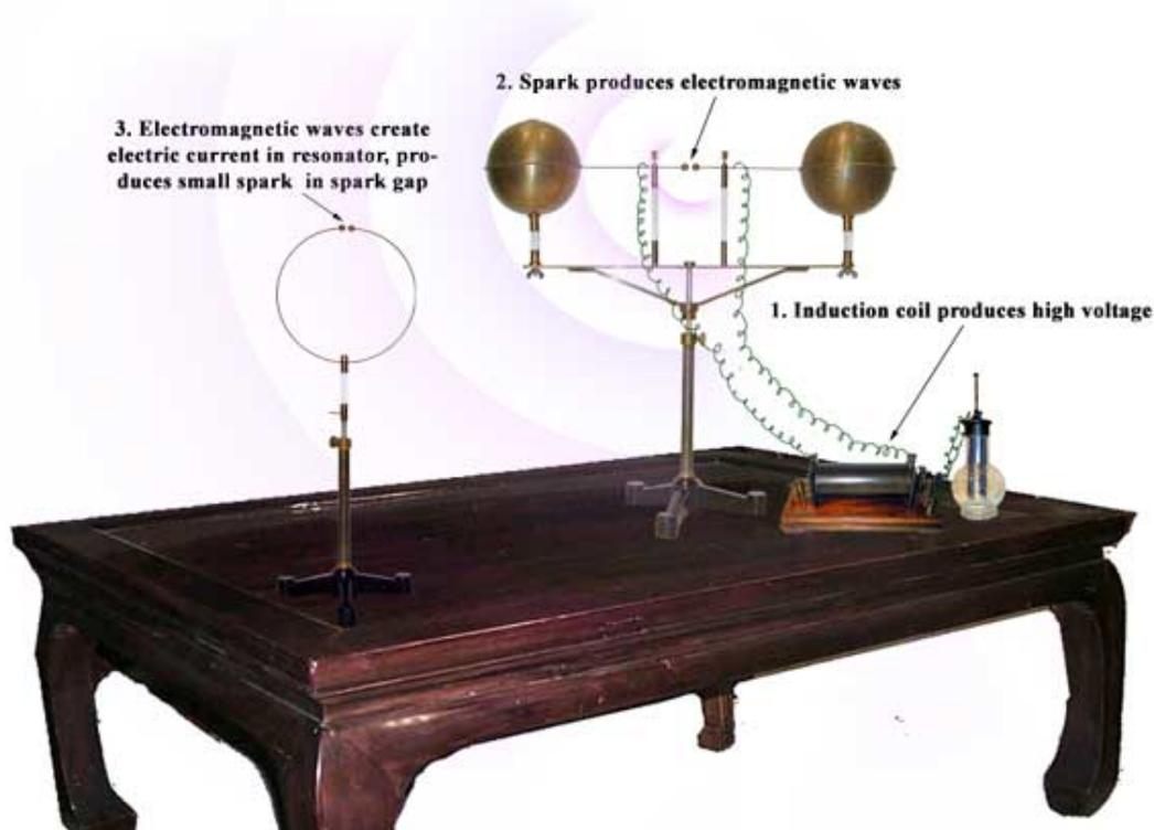
The ring at the left detects the waves. The ring is not completely closed: there is a small gap. The waves cause small sparks to be seen jumping the gap. If the ring is turned ninety degrees, you don't see the sparks, showing that the waves are "transverse waves",
